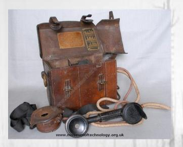
On the left a WW1 telephone used in the trenches. Radios were still not available so long cables had to be strung between the trenches and headquarters.
